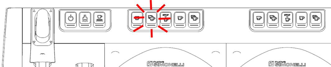
LED 1 LONG COFFEE = SERIAL CONNECTION (DIRECT CONNECTION)
