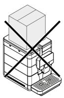
⚠ Due to the total weight, do not stack more than three machines on top of each other. The machine should be stored in its original packaging, in a dry and/or dust-FREE place.
