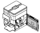
Remove the brew group by pulling it by the handle and pressing the «PRESS» button.
