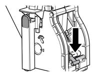
Make sure that the hook which locks the brew group is in the correct position. firmly press the "PRESS" button to check its position.
