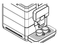
Push the dispensing spout towards the machine interior to its limit stop, to allow the use of tall glasses or MUGS. In this case, you can just brew one product at a time.
