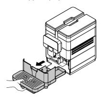
After emptying it put the drip tray back into place. Select "OK" and press the "OK" button.
