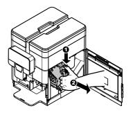
Wash the brew group with lukewarm water; carefully wash the upper filter. Before placing the brew group in its seat, ensure that there is no water left in the brewing chamber.
