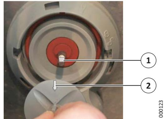
Fig. 45: Fitting the mixer impeller
