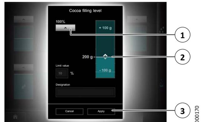
Fig. 12: Adjusting filling levels more accurately
