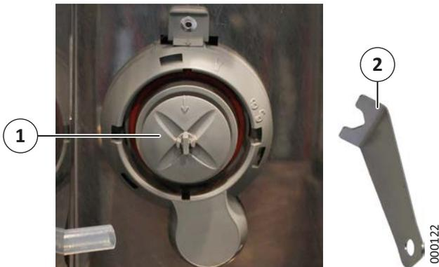
Fig. 44: Removing the mixer impeller
