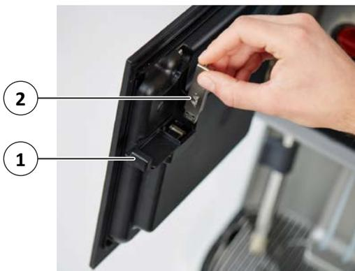
Fig. 36: Inserting the USB stick
