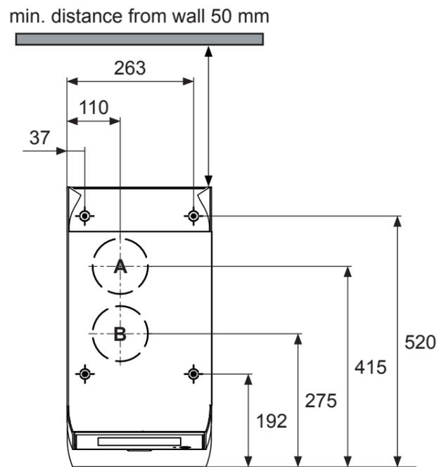
A  $\varnothing$  120 for lines (does not apply to machines with MCU30)
