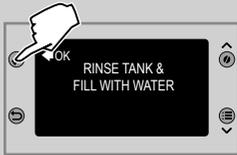
**10** The message indicates the end of the first step. The water tank needs to be rinsed. Fill the water tank with fresh water up to the MAX level. Press the “✓” button.
