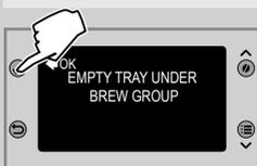
5 Empty the drip tray (internal) / (external). Press the "✓" button.
