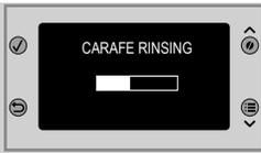
**16** The machine starts dispensing water from both the coffee dispensing spout and the milk dispensing spout. The bar shows the cycle progress.
