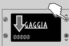
**1** To temporarily change the amount of ground coffee, press the "☉" button on the control panel.
