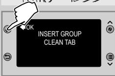
**5** Put a "Coffee Oil Remover" tablet in the pre-ground coffee compartment. Press the "✓" button.
