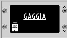
**6** When the operations described above have been completed, the machine shows this display. The 100% AquaClean icon appears on the machine-ready screen to indicate that the filter has been activated.
