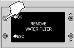
4 Remove the water tank and the AQUACLEAN water filter (if any).
