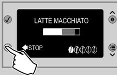
8 Once the milk froth has been dispensed, the machine brews coffee. Brewing can be stopped earlier by pressing the "↶" button.
