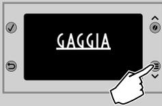
1 Press the “☰” button to access the machine main menu.
