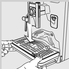
**4** Insert the (external) drip tray with grill into the machine. Make sure it is correctly placed.
