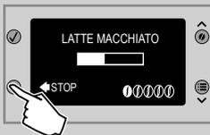
7 When this screen is displayed, the machine starts dispensing frothed milk. Dispensing can be stopped earlier by pressing the "↶" button.
