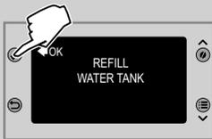
**12** When the machine stops dispensing, fill the tank with fresh water up to the MAX level. Press the “✓” button to confirm.
