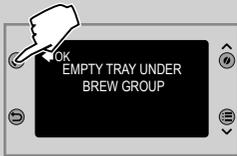
**11** Empty the (internal) drip tray and place it back, then press the “✓” button.
