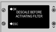
**2** The display indicates that you need to descale the machine before activating a new filter. Press the “✓” button to start the descaling procedure.
