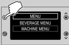
2 Select MACHINE MENU by pressing the “∨” or “∧” scrolling button. Press “✓” button to confirm.
