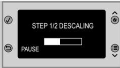
**9** The machine will start dispensing the descaling solution at regular intervals. The bar on the display shows the cycle progress.
