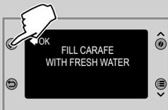
**14** Wash the milk carafe thoroughly and fill it with fresh water. Insert the milk carafe into the machine. Press the “✓” button to confirm.
