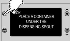
**6** Place a container (1.5 l) under the coffee dispensing spout. Press the "✓" button to start the cleaning cycle.
