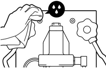
For thorough maintenance, we suggest you use the Lelit brush (code PL106 - not included), which will help you clean the nozzles and the spaces between the gaskets more effectively, removing stains and coffee residues from even the smallest cracks.
