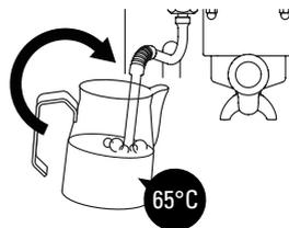
Insert the wand all the way down and tilt the jug to create a vortex. Heat the milk to the desired temperature, without exceeding 65°C. *Close the steam.*
