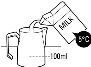
Fresh whole milk provides a smoother, creamier and tastier froth. Milk will not froth at over 65°C, so cold milk from the fridge should be used to allow more time for it to froth. The best jugs to use are made of stainless steel and have a spout, like the Lelit jug (code PL101-PL102 - not included).
